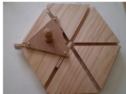
Figure 9: A trammel with 3 slots.
